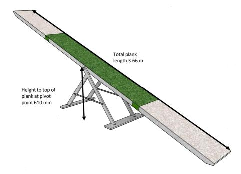
The see-saw will consist of a plank firmly mounted on a central bracket. The length of the plank must be 3.66m. The width must be between 295mm minimum and 305mm maximum. The height at the pivot point must be 610mm from the ground to the top of the plank.
