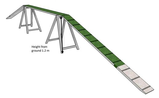
A walk plank of 1.2m measured from the ground to the top of the plank, with firmly fixed ramps at either end. The planks must be 3.66m in length and a minimum of 254mm and a maximum of 305mm in width.
