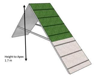
The A frame must comprise of two ramps, 2.74m long by 914mm wide, hinged at the apex 1.7m from the ground. The last 1.067m from the bottom of each ramp should be a different colour to indicate the area with which the dog should make contact. Each ramp to have a non-slip surface, and anti-slip slats at intervals but not within 152mm of the start of the contact area.
