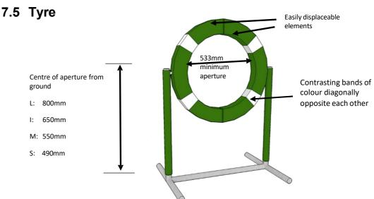
The aperture centre of the tyre from the ground must be:
