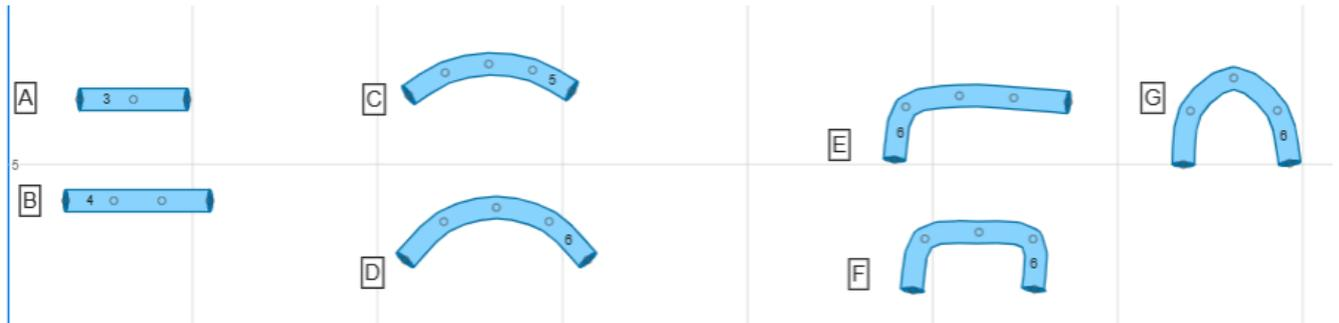
A and B: 3m and 4m tunnels have 0° angle and must only be used straight
